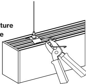
19. Secure power feed cable to suspension, cable every 3 inches using cable ties (cable ties provided by others)
