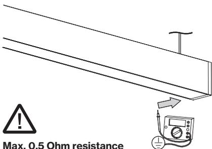
27. Connect inset(s) wiring, grounding clip and fall protection to channel(s)
