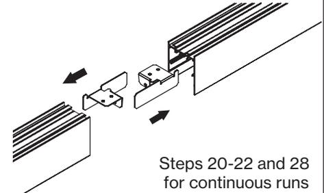
21. **SYSTEMS:** Use screws to secure connectors to channels
