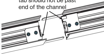
22. **SYSTEMS:** Slide channels together. Secure connectors with screw and nut.
